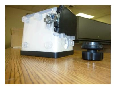
3. Release both (left and right) toggle latches from the catch plates in order to remove the front window.
