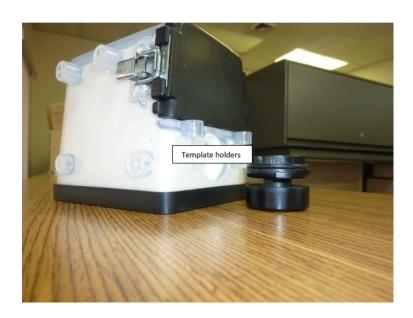
2. Remove the knob at the probe input channel by rotating it counterclockwise.
