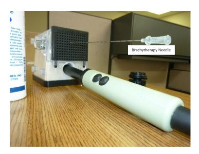
7. Insert the brachytherapy needle through the template holes and follow up its path using theultrasound planes (Transverse or Sagittal). Probe Brachytherapy Needle
